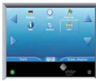
A colour graphic screen with 7 touch-sensitive sections allows easy operation by using a menu structure to access the data. Thanks to the built-in web server, this can also be done remotely when a network connection is available.
