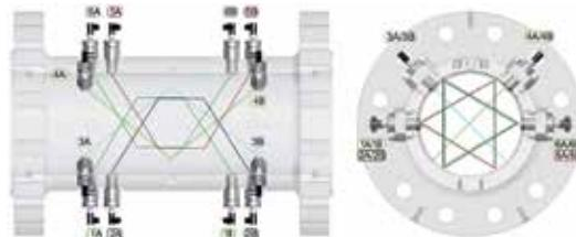
The Q.Sonic<sup>plus</sup> uses two pairs of double and two single reflection paths. Taking the mean value of both pairs will result in a symmetrically weighted measurement.
