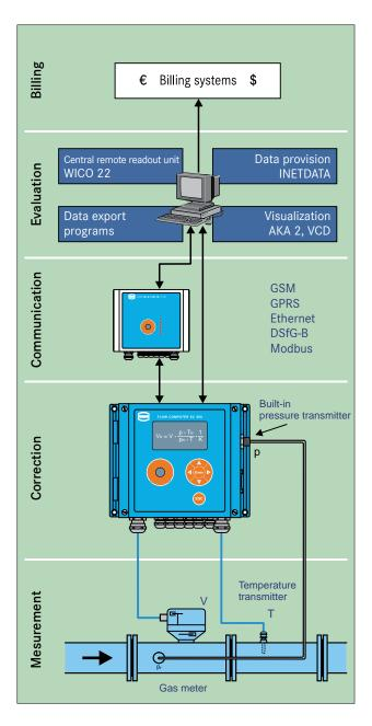
A much more convenient way of operating the EC 900 is by using the Dialog 900 program for reading out, parameterizing and visualizing data, which is supplied together with the device. This program can be used both locally and in the central unit. It is also suitable for operating the MRG 905 and MRG 910 measured-value recording devices.
