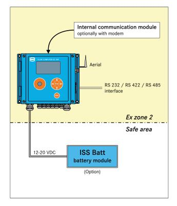
The EC 921 version is intended for use in Ex zone 2; it is not permissible to operate this device in Ex zone 1. It is supplied by two lithium batteries as standard: one for the corrector and the other for the internal communication module.
